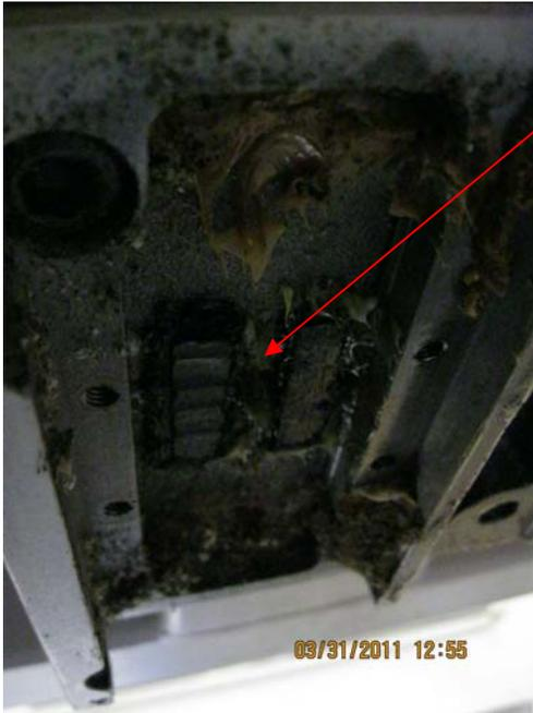
Note: Debris or solidified grease packs behind the bearing as shown and stops flow of new grease into bearings especially if incorrect grease has been used.
